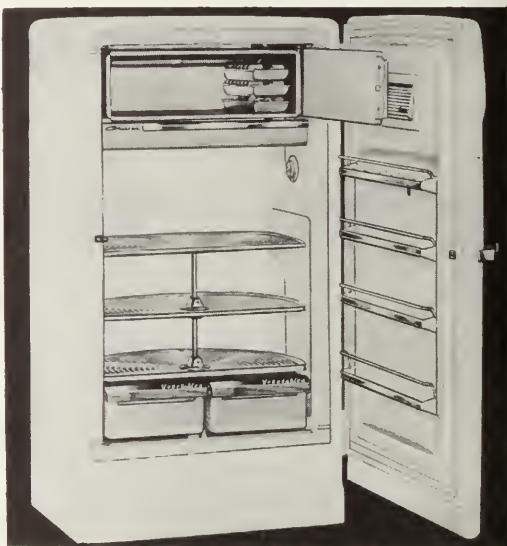
9-7. A refrigerator cabinet with revolving shelves. The center post permits the shelves to revolve and also enables the shelves to be adjusted for height. (General Electric Co.)
